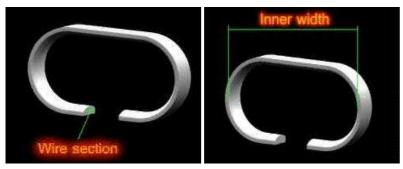
Height of bow: It should be as low as possible for stable running of traveller. It should also have sufficient yarn pasage.
